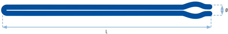
Bandsplinte, gespalten (Open End Pins) Split bracelet pins (Open End Pins)
